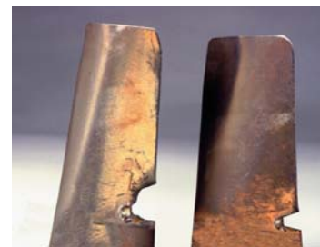
Severely damaged turbine blades seriously affect power output.
