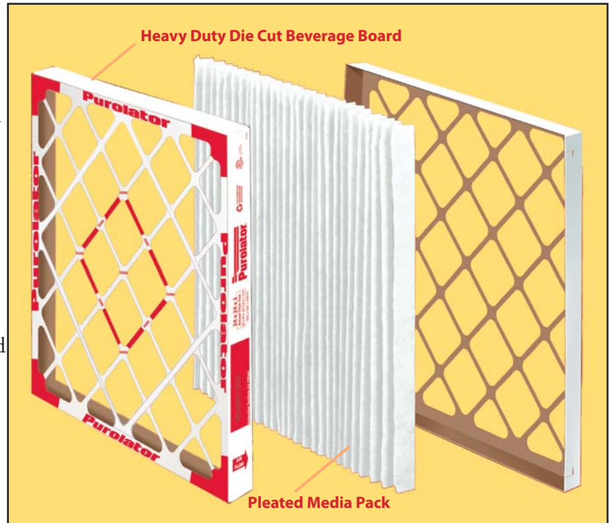
Two mating pieces of die cut beverage board form a double wall frame around all four edges of the filter. Hi-E 40HC filters will not rack or warp under normal operating conditions.
